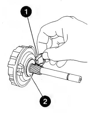
COMPONENT CHECKING AND REPAIR Checking planetary gear train Further disassembly: Pull drive shaft (1) out of intermediate bearing (2). Pay attention to TX collar (3).
